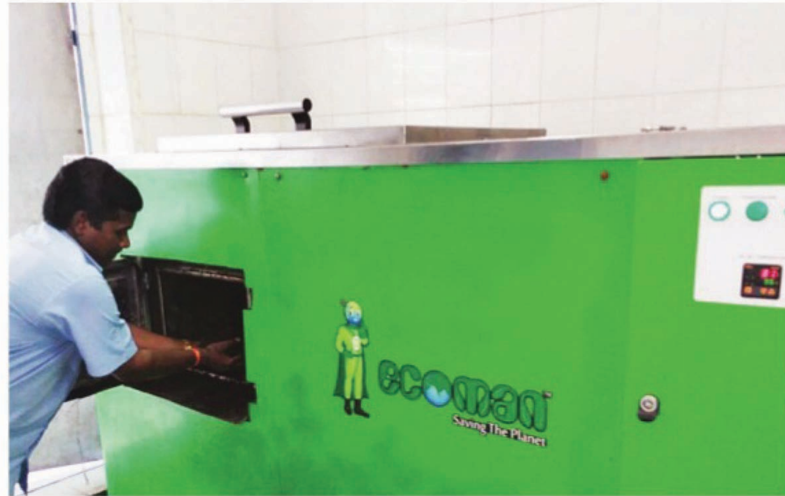
A hotel using on-site composting machinery to turn organic waste into manure
